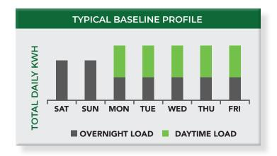
For the first time, it's easy to see how much energy is consumed during non-operational hours. For many commercial buildings, almost 40% of plug load expense occurs when the building is empty.
